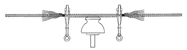
FOR TOOL APPLICATION, INSERT HALF OF THE REINFORCEMENTS IN ONE CAVITY AND ENTER THE OTHER HALF IN THE OTHER CAVITY OF THE OPEN WRENCHES, KEEPING THE ENDS EVEN. HOOK WRENCHES OVER THE CONDUCTOR AND CLOSE JAWS. SPACE WRENCHES APPROXIMATELY ONE REINFORCEMENT PITCH APART AND TWIST THEM IN THE SAME DIRECTION AS THE LAY OF THE CONDUCTOR. WIND EACH WRENCH TO THE END OF THE REINFORCEMENT AND REMOVE.
