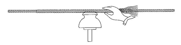
FOR HAND APPLICATION, HOLD ONE OR MORE REINFORCEMENTS AGAINST THE CONDUCTOR WITH MIDPOINT AT THE INSULATOR, AND ROTATE IN SAME DIRECTION AS THE LAY OF THE CONDUCTOR, FOR THREE OR FOUR INCHES EACH SIDE OF CENTER. IN LIKE MANNER APPLY REMAINING REINFORCEMENTS TO CENTER SECTION. AFTER ALL HAVE BEEN STARTED, COMPLETE THE APPLICATION BY A ROTARY OUTWARD WIPING MOTION OF THE HAND. MAKE CERTAIN THAT THE ENDS SNAP INTO PLACE IN PROPER ORDER.
